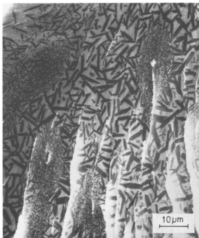
Figure 6 Fibrillar structures of the second phase found in polypyrrole grown on mild steel
